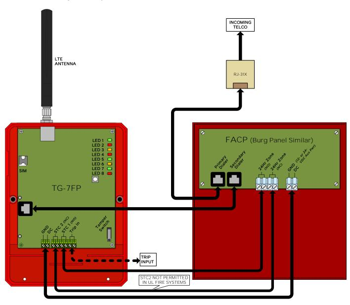
For all UL/ULC Commercial Burglary Installations, a Tamper switch must be wired to monitor the TG-7FP enclosure. The wiring from Tamper Switch to the panel shall be in a rigid or flexible metal conduit along with other wiring from the TG-7FP to the Panel.
